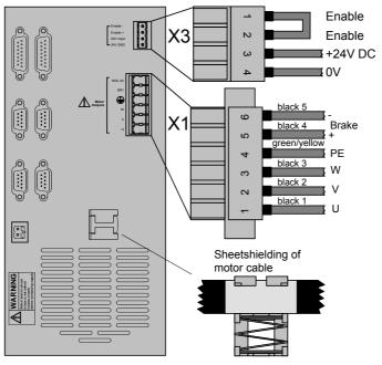
Note the screened connection of the motor cable on the lower side of the unit.
